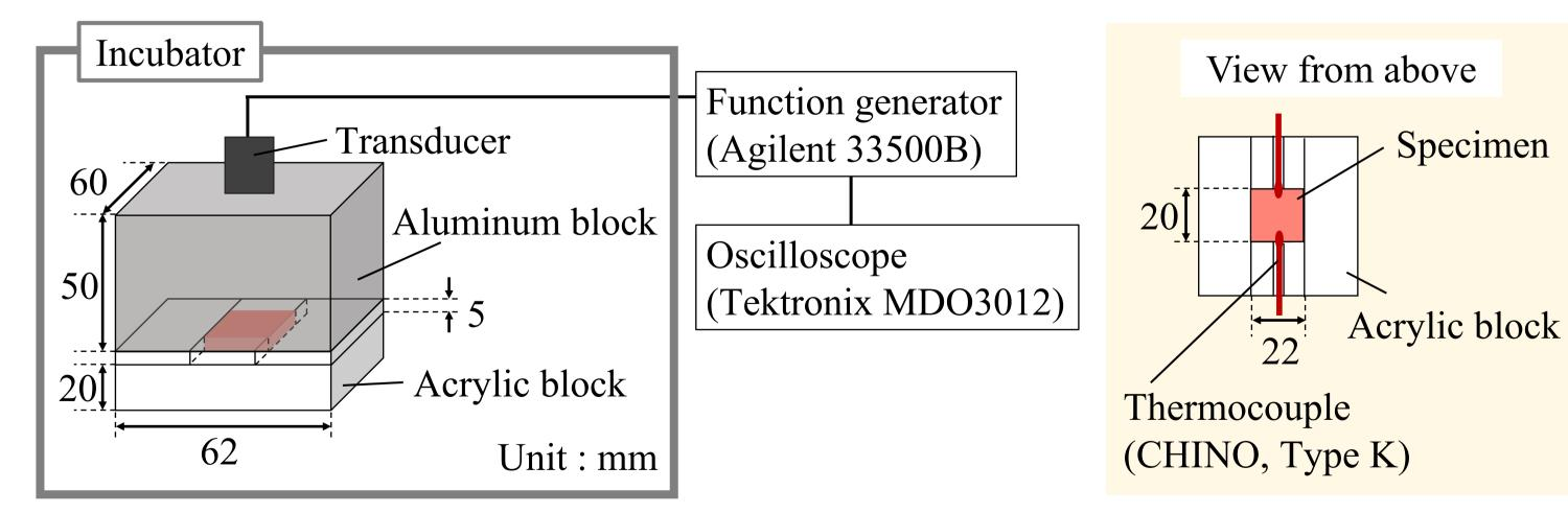
The thickness and the flatness of a specimen are ensured by the depth of depression and the surface of aluminum and acrylic block.
