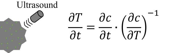
$\partial T/\partial t$  Rate of temperature rise  $\partial c / \partial t$  Rate of sound velocity change  $\partial c / \partial T$  Temperature coefficient of sound velocity
